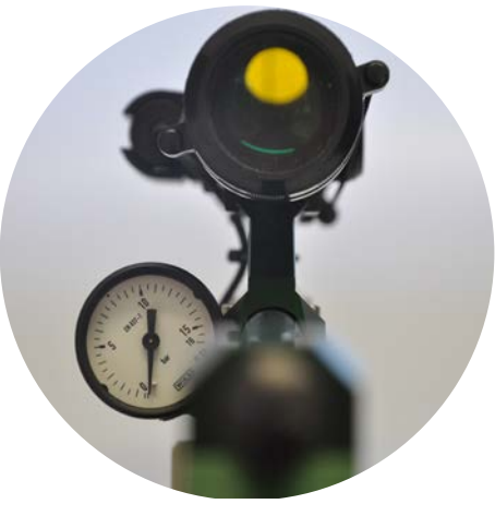
The pressure dial as viewed by the operator, with the telescopic sight above and the laser to the left hand side.
