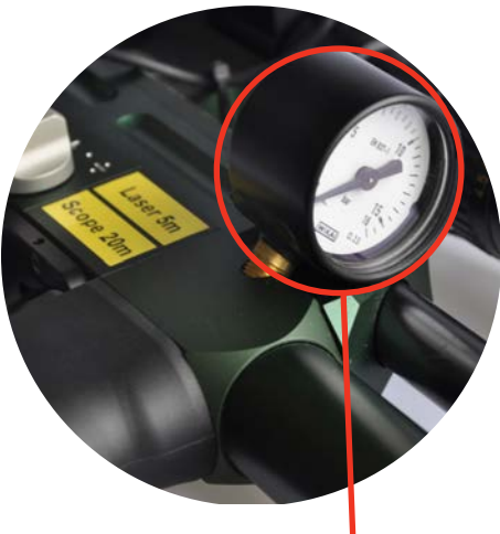
The pressure dial is located adjacent to the CO 2 adjuster, just above the trigger. Note this is the 16 bar model.
