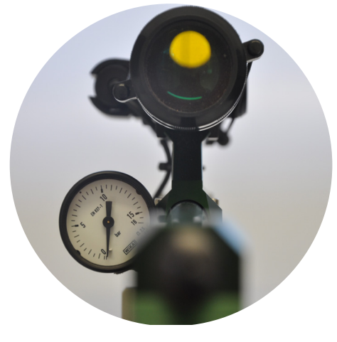
The pressure dial as viewed by the operator, with the telescopic sight above and the laser to the left hand side.
